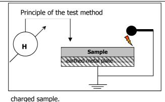
The sample is located on an earthed metal plate.
